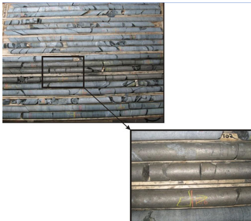
Figure 23: Drill core from hole HN-08-07 from Southampton's 2008 drill program showing large blebs of pyrrhotite, pyrite and chalcopyrite within massive sulphide
